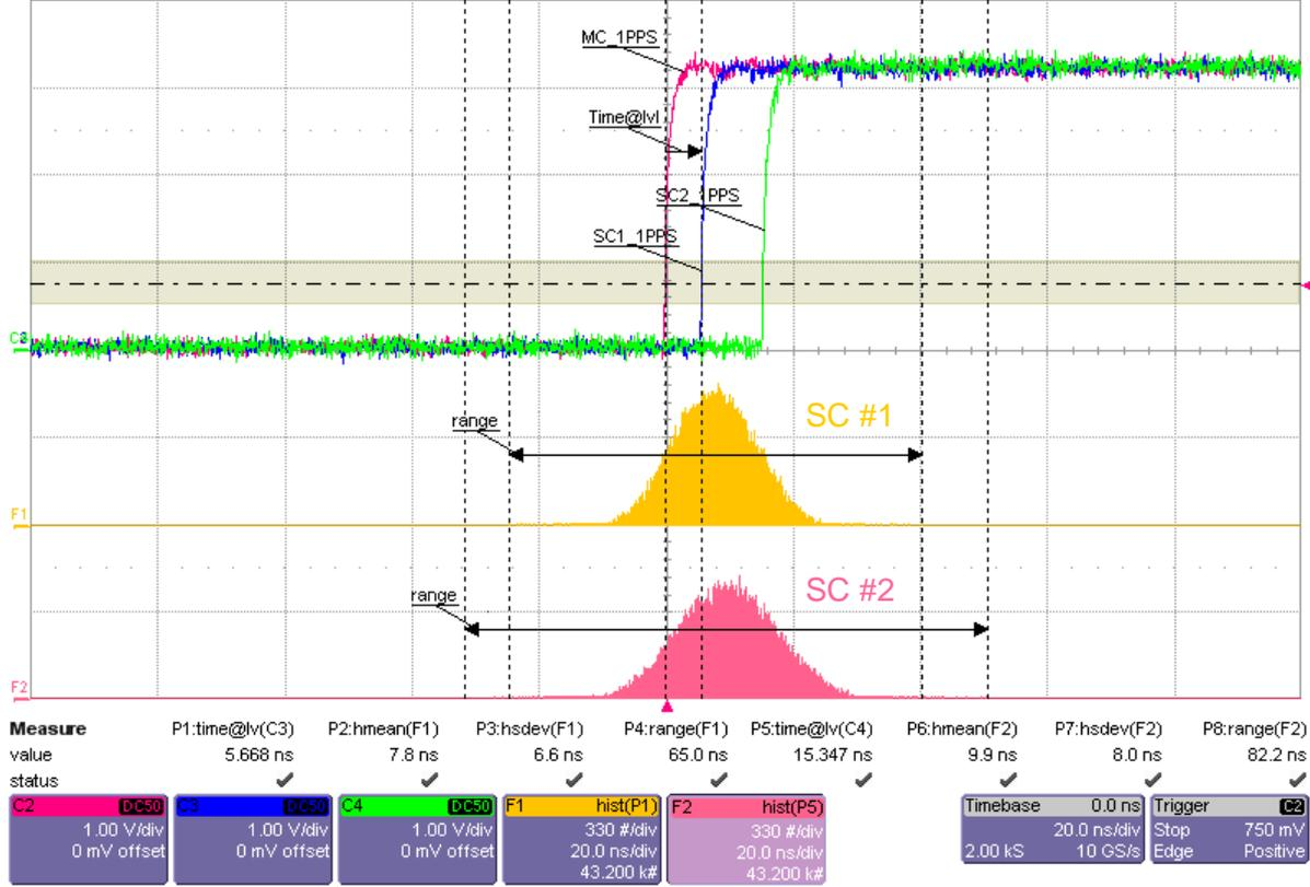
Figure 9: Cascaded TC measurement without traffic
