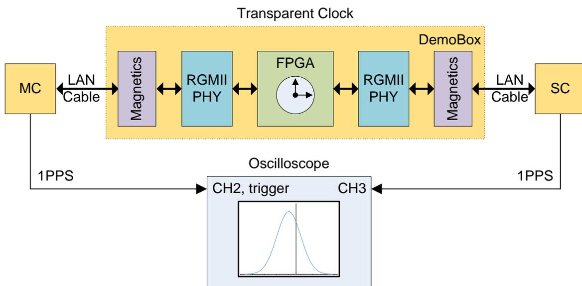
Figure 6: Single Transparent Clock test setup
