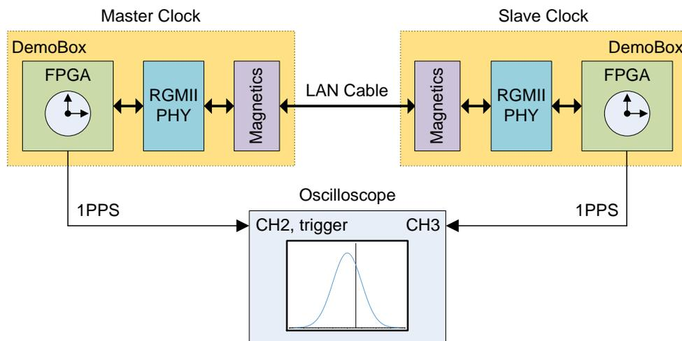
**Figure 4:** Directly connected Master and Slave Clocks test setup
