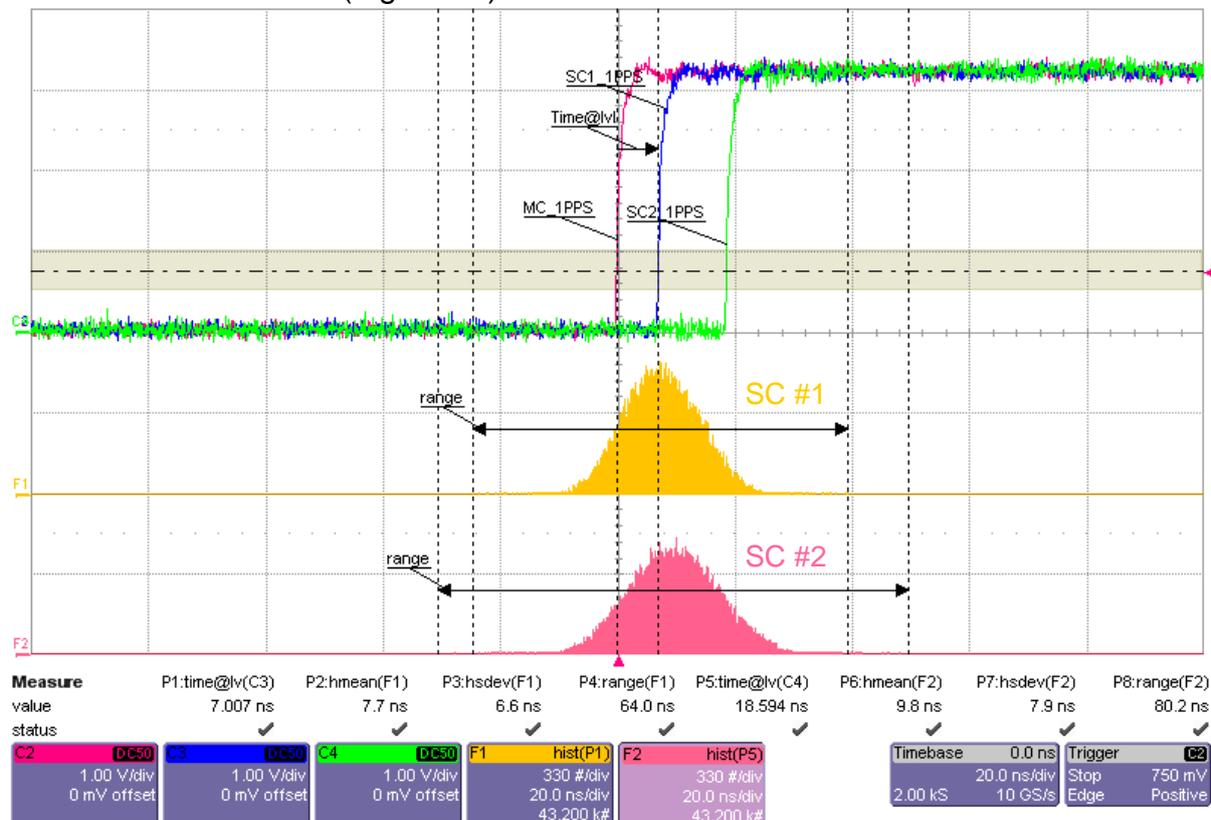
**Figure 12:** One Sync message per second measurement without traffic
