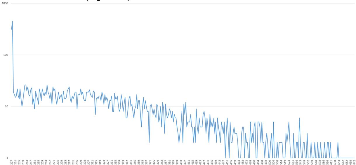
**Figure 11:** Correction field value distribution of 3,600 Sync messages with 80% additional network traffic
