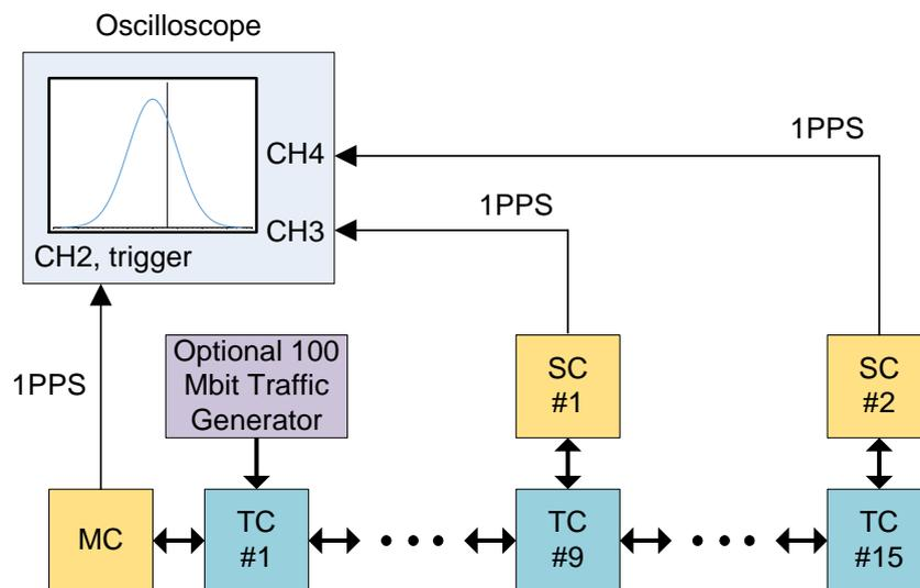
Figure 8: Cascaded Transparent Clocks test setup
