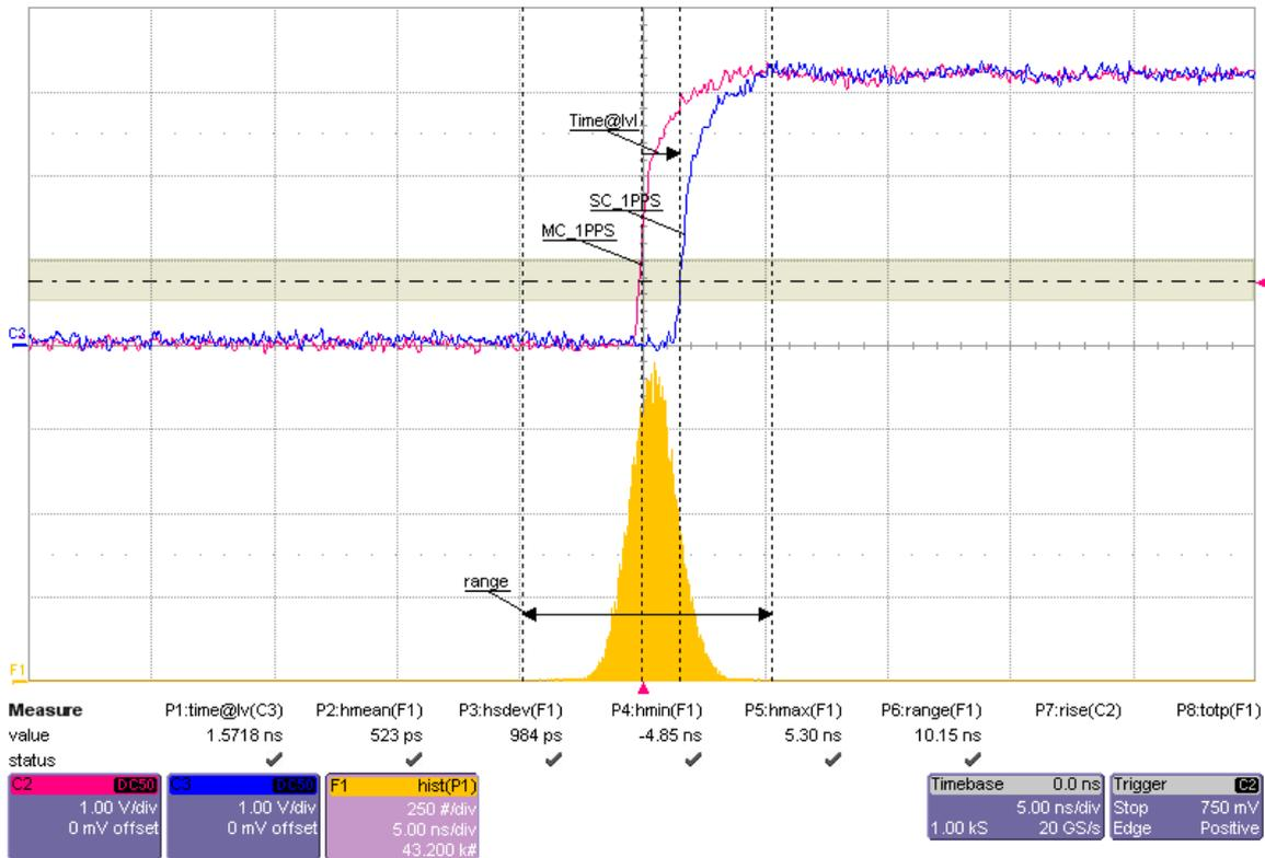
Figure 5: Directly connected clocks measurement
