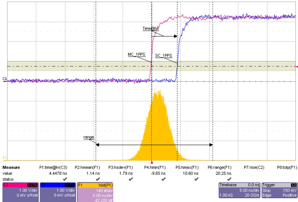
Figure 7: Single Transparent Clock measurement
