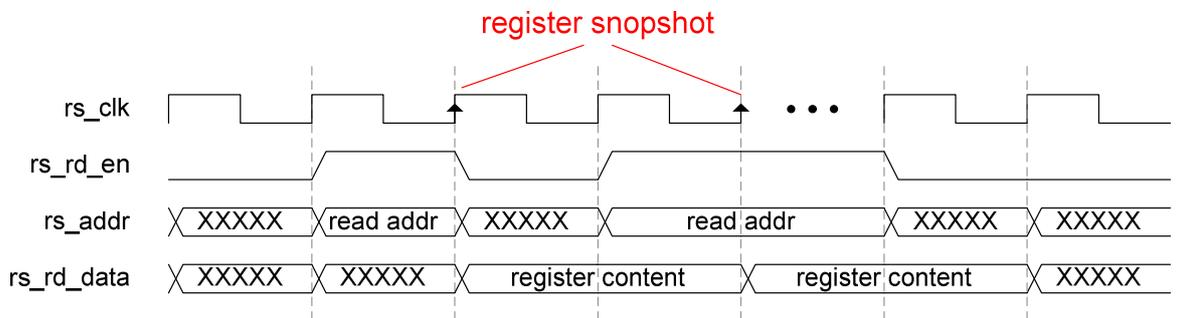
**Figure 12: Register Set read cycle timing**
