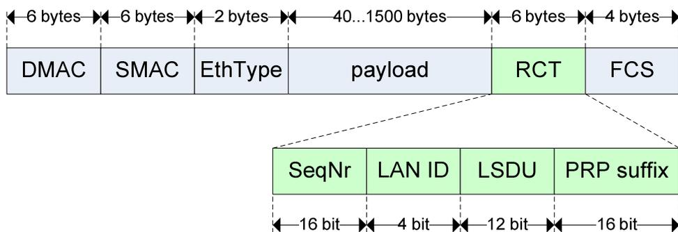
**Figure 4:** Structure of a PRP-tagged frame
