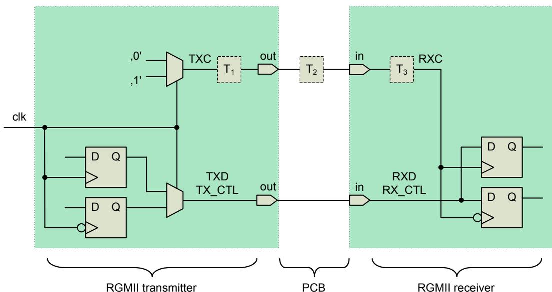
**Figure 15:** RGMII signal path diagram
