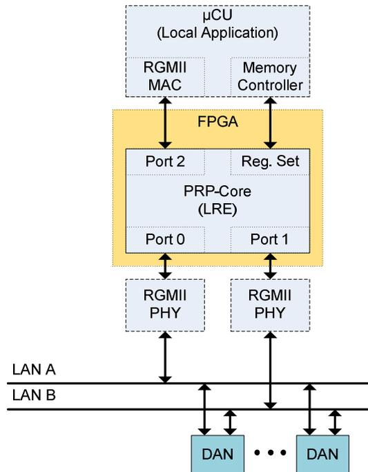
**Figure 9:** Dual Attached Node (DAN) use case
