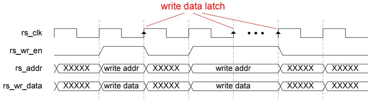
**Figure 11: Register Set write cycle timing**
