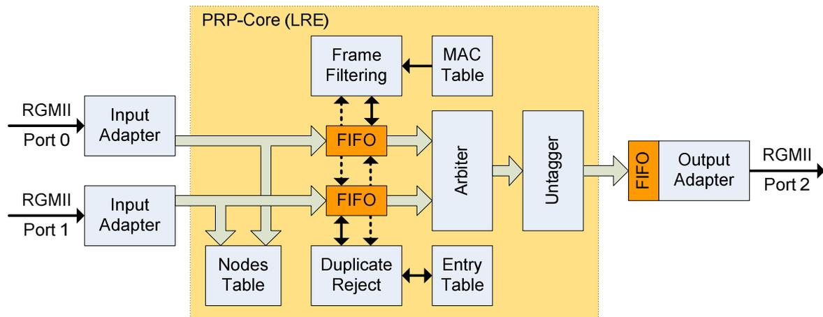
**Figure 5:** PRP-Core receive path block diagram
