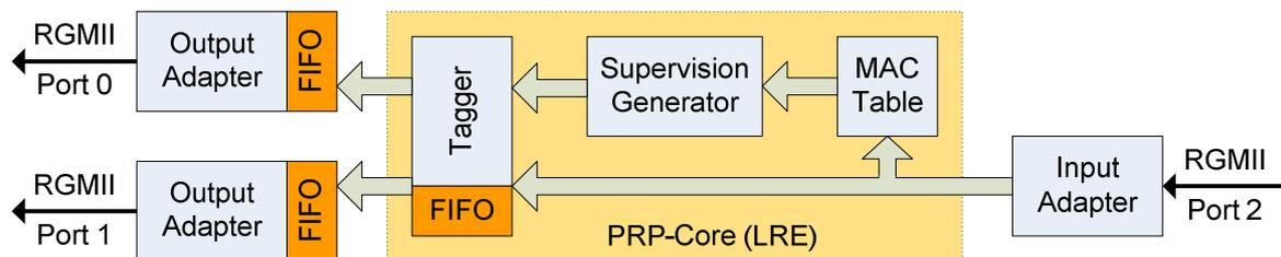
**Figure 6:** PRP-Core transmit path block diagram
